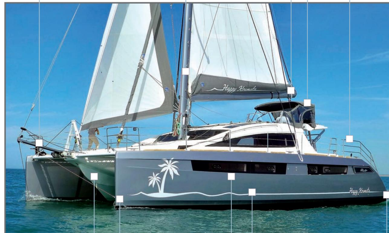
Protected from impact by a wave-piercing wing, the superstructure reinforces the forward beam, simplifies the anchoring station and creates the original distinctive Privilège living space
